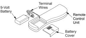
Figure 40 - Installing Battery in Hand-Held Remote Control Unit (GHRCTB Series)
